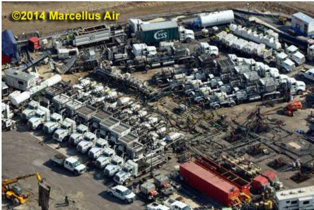
Figure 18 – Frac array with 2,500 horsepower pumps running 24-7 to crack the shale
